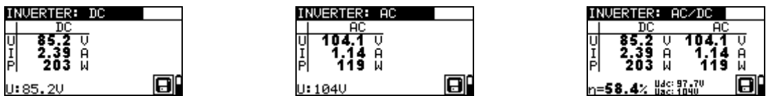
Figure 5.23: Examples of PV inverter test results screens - 1 phase a.c. output
