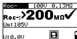
Figure 5.4: Examples of insulation resistance measurement result
